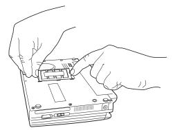
Sample inserting the memory module into the slot
